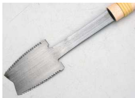
▲ Both edges have a convex curve, which makes them ideal for starting a cut in the middle of a panel
